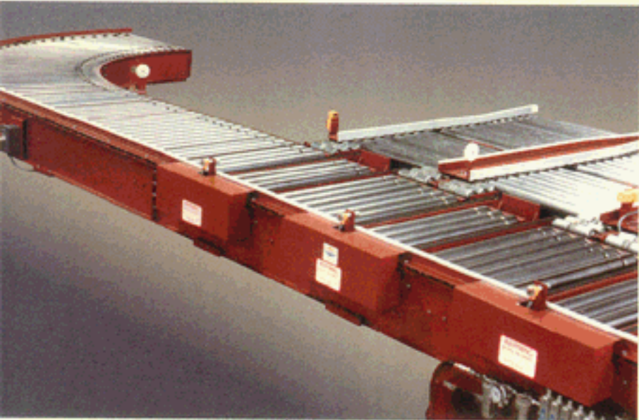
Pop-up "V" belt transfers move product from main line to side spurs for major appliance manufacturer
